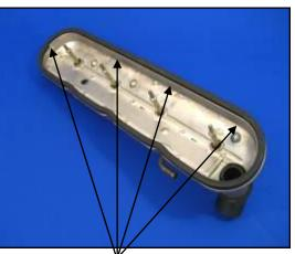
THOURGHLY CLEAN SURFACE SOAK SEAL IN HOT WATER TO MAKE MORE FLEXIBLE. START WITH THE JOIN AND WORK AROUND FIT SUPPLIED NUTS TO BOTTOM OF ROCKER COVER MOUNTING BOLTS AND TIGHTEN
